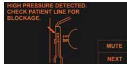
High Line Pressure Alarm Screen
